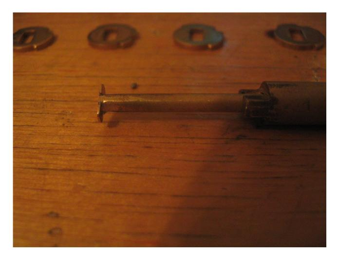
Here is a close-up of the tip of the Abus Plus pick. The key-shaped piece at the left end of the tool is 0.5 millimeters thick and is made from flattened piece of brass tubing and soldered to the shaft with lead-free solder. I don't go into details about the pick tool, because we'll need only the tip part of the tool and I might make a different PDF document about the manufacturing of the pick tool.
