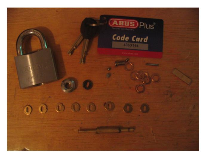
In the above picture can be seen the Abus 88/50 padlock that costs about 20-25 Euros. It is equipped with the Abus Plus cylinder, that is a rotating detainer disc style cylinder. The code card shows a number sequence 4363144. The code corrsponds to the cuts in the key such that number 6 cut is a no-cut and number 1 is a fully cut. The numbers correspond to the cuts from bow to tip.
