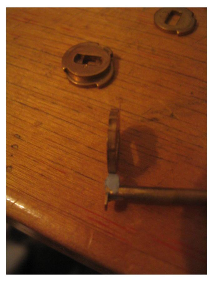
The thickness of the Blu-Tack plus the pick tools end should not exceed that of the detainer disc. This is because the pick tools end still has to have room to turn in the lock. In the above photograph the Blu-Tack is a little too thick.
