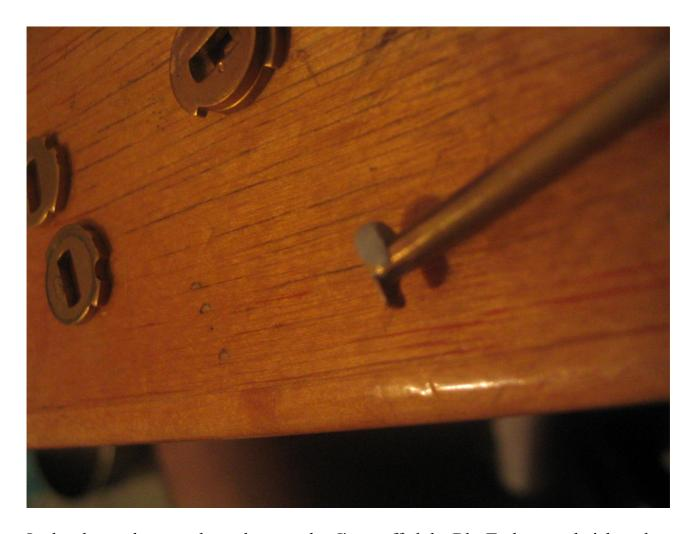
In the above photograph can be seen that I've stuffed the Blu-Tack around pick tools end on the "user" side. I only applied it to the other part of the pick tools end, but it can be applied to both sides. This way it'll give stability in the lock and you don't have to think about at which side of the detainer disc the stamped number was.
